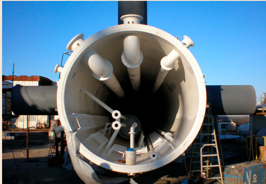
Skim pile vessel in fabrication for Offshore West Africa project
