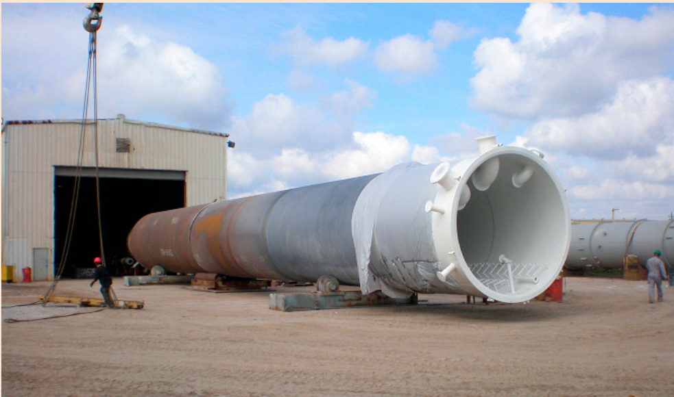
Large 12' x 120' vertical vessel for storm water run off
